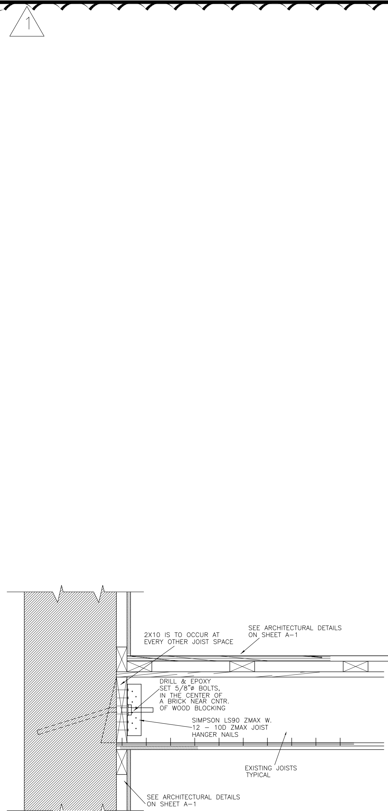
1 S-4 FLOOR DETAIL AT EXT. WALL, PERPENDICULAR 1 1/2" = 1'-0"
